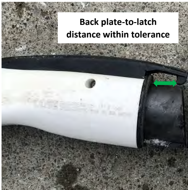
Figure 30. Example J1772 connector plate-to-latch tolerance
